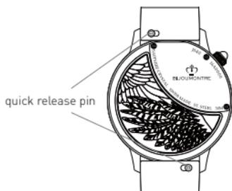
Your watch is equipped with quick release pin for strap and metal bracelet changing.
